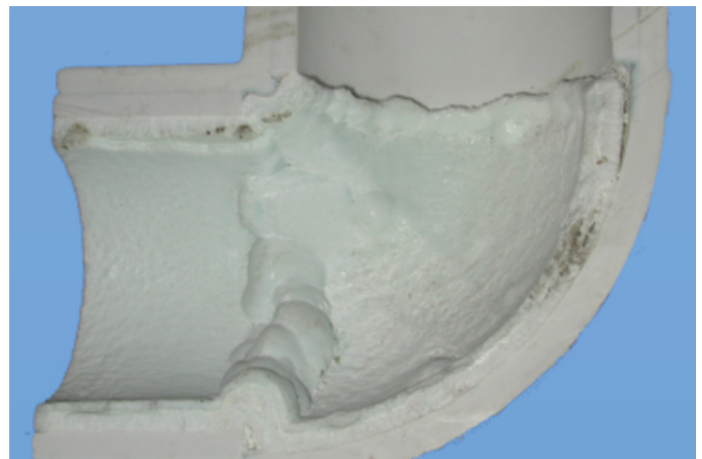
Scale in pipes can lead to reduced flow and create unwanted turbulence
